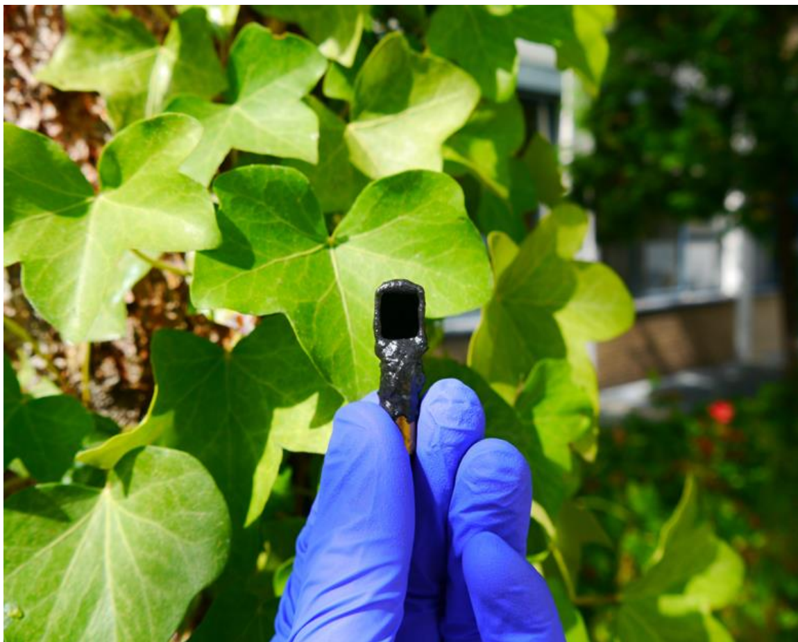
Fig. 1: The small cell sets a record in efficiency by converting 14% of the incoming sunlight into hydrogen.
