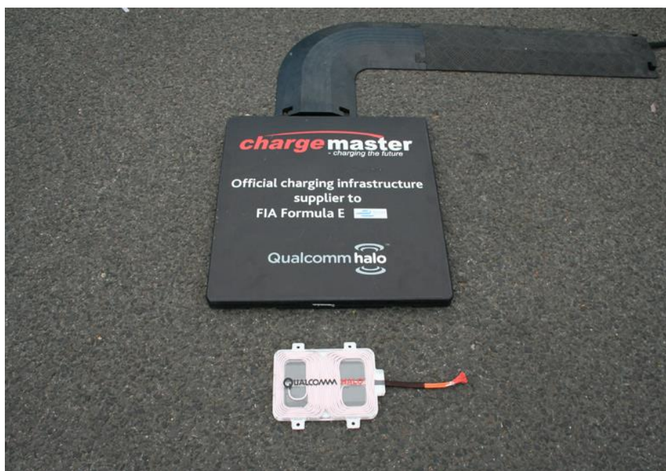
Fig. 3: Primary and secondary coil of a Formula E Medical Car
