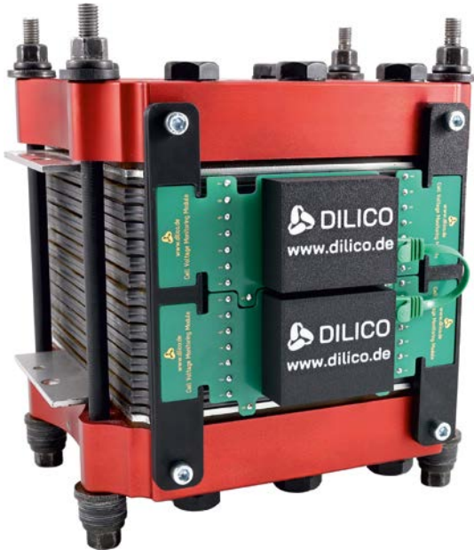
Dilico's cell voltage pickup converts the measurements directly on the stack into digital data. © Dilico
