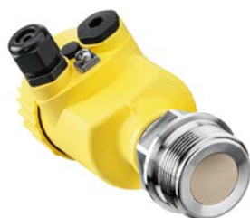
For pressures up to 100 bar, dry ceramic-capacitive measuring cells have proven themselves.
