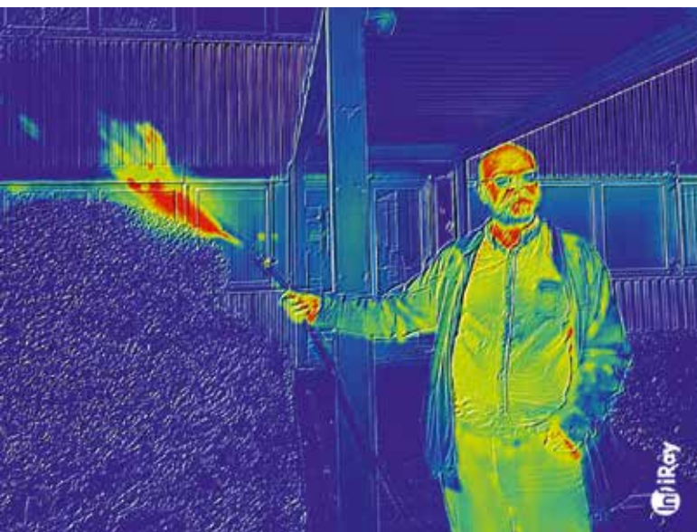
Fig. 2: Peter Pioch from WBZU shows an H 2 flame with a thermal imaging camera [Source: WBZU]
