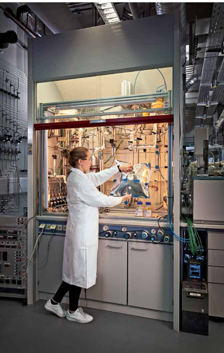
Fig. 1: Retrieving high-purity hydrogen from an LOHC system [Sources: Allgemeine Services KIT, Bramsiepe]
