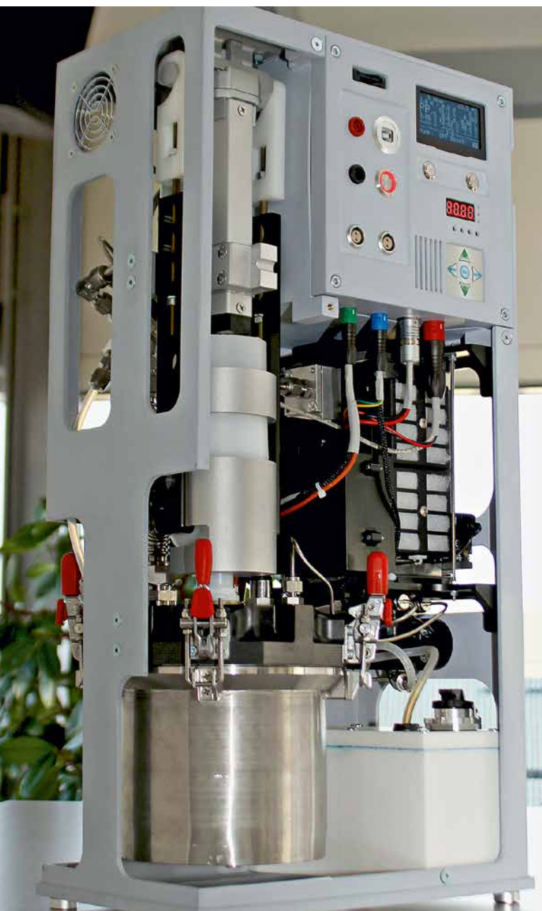
Fig. 3: Compact and portable 100-watt power generator that uses hydrolysis to generate electricity [Source of all images: IFAM]
