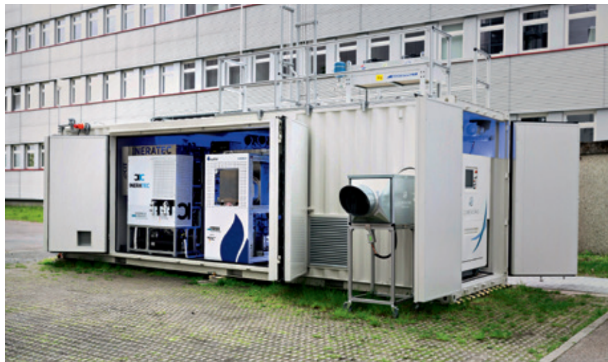
Fig. 2: This compact power-to-liquid pilot plant put up at Karlsruher Institut für Technologie – KIT synthesizes fuel from carbon dioxide in the air. [Source: Sunfire]
