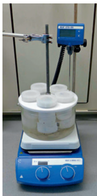
Fig. 1: Test setup, including 5 sample containers, to initiate an ex-situ Fenton's reaction. [Source: Fraunhofer ISE]
