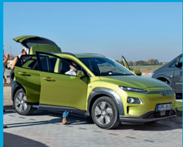
Fig. 3: One difference between the Kona Electric and any Kona with an internal combustion engine is the lack of a radiator grill in the front.
