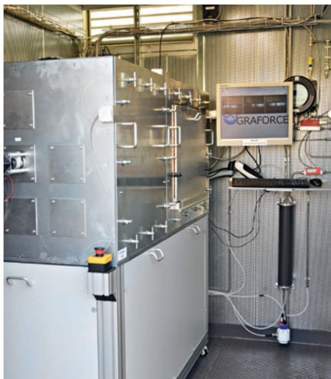
Fig. 2: The silver boxes (left) contain three receivers, whose interior, including the blue shimmering plasma, is shown on screen.
