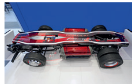
Fig. 3: Prototype of a hydrogen drive that FPT is developing for Iveco. [Source: FPT]
