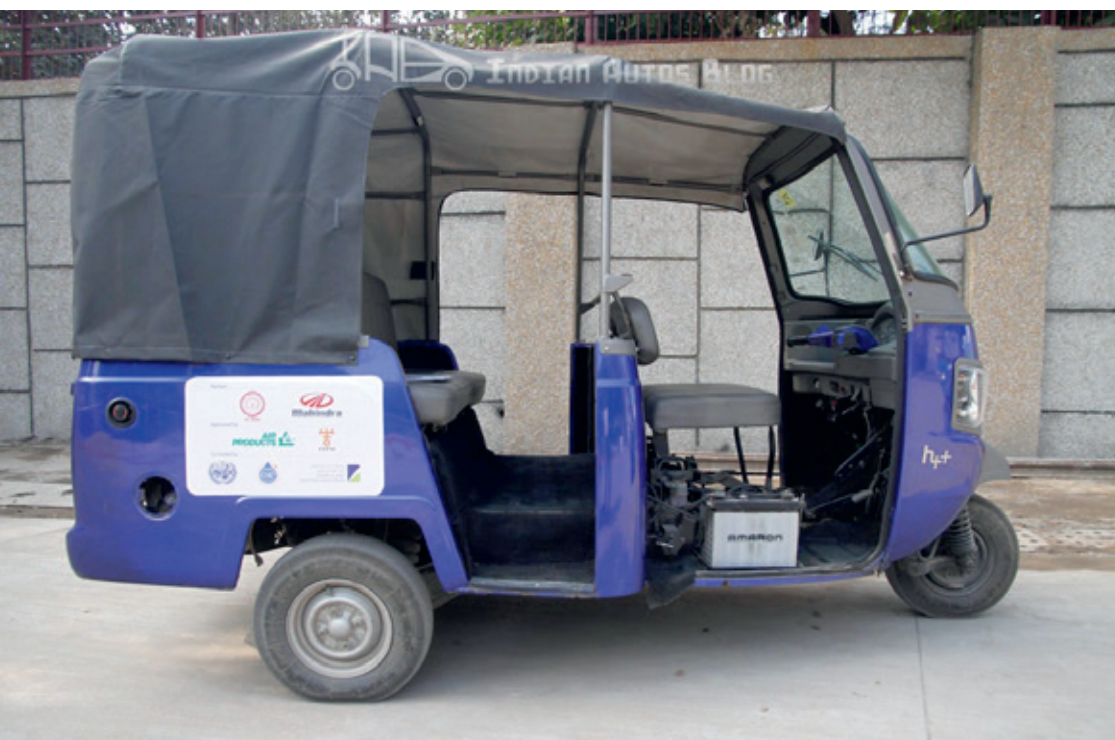
Fig. 1: Three-wheeled electric rickshaw HyAlfa by Mahindra
