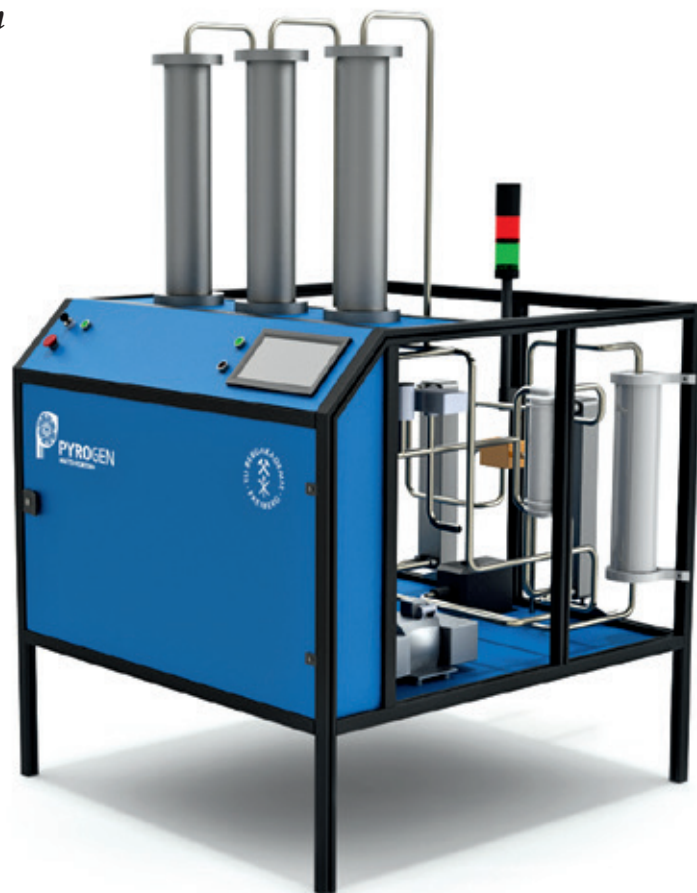
Fig. 1: Demonstration system to produce hydrogen based on pyroelectric materials
