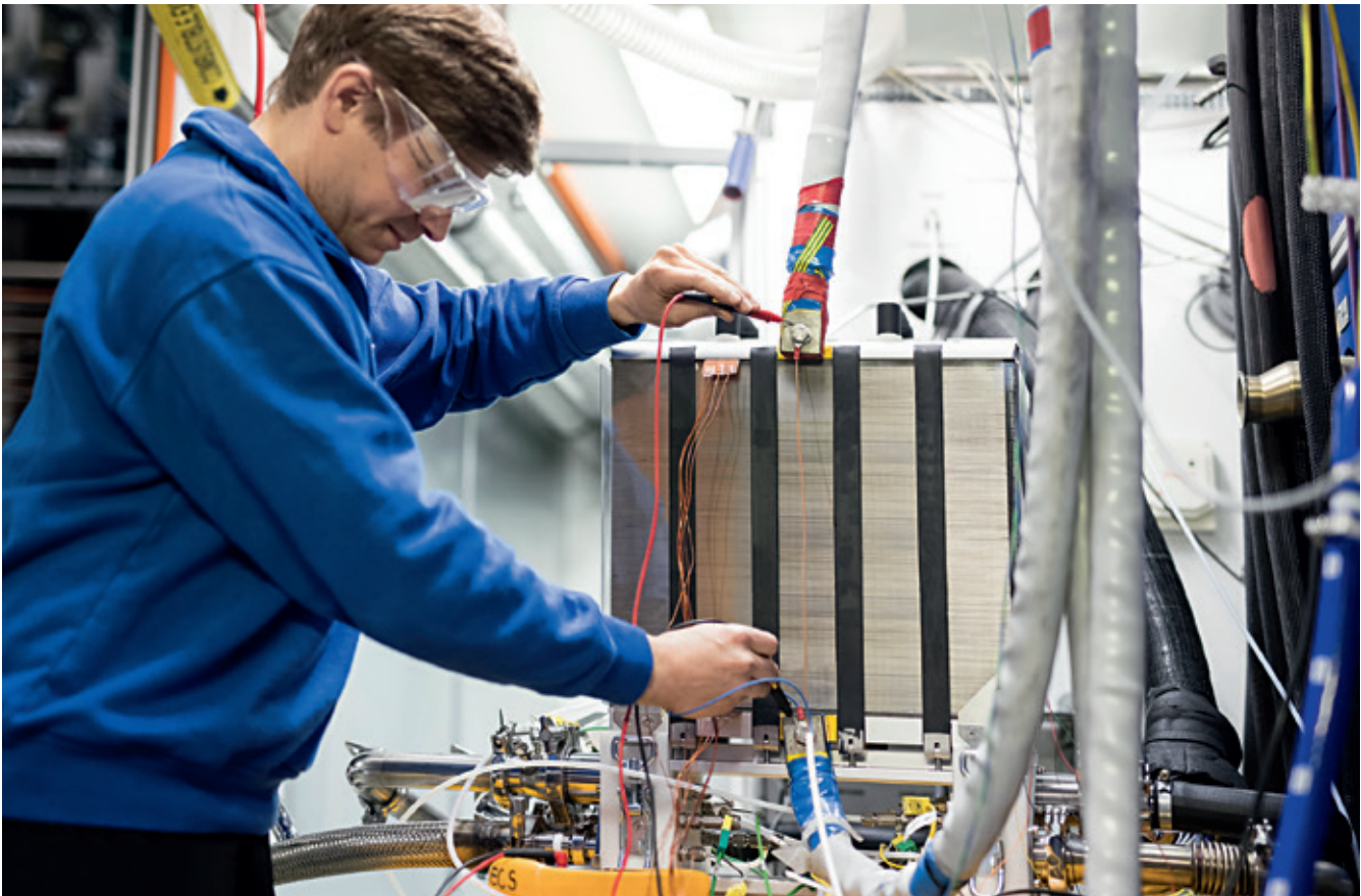
Fig. 2: Test stand for Evolution 1 stack
